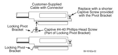
3. Insert the bottom edge of the locking pivot bracket inside the lower edge of the rear panel cutout.
